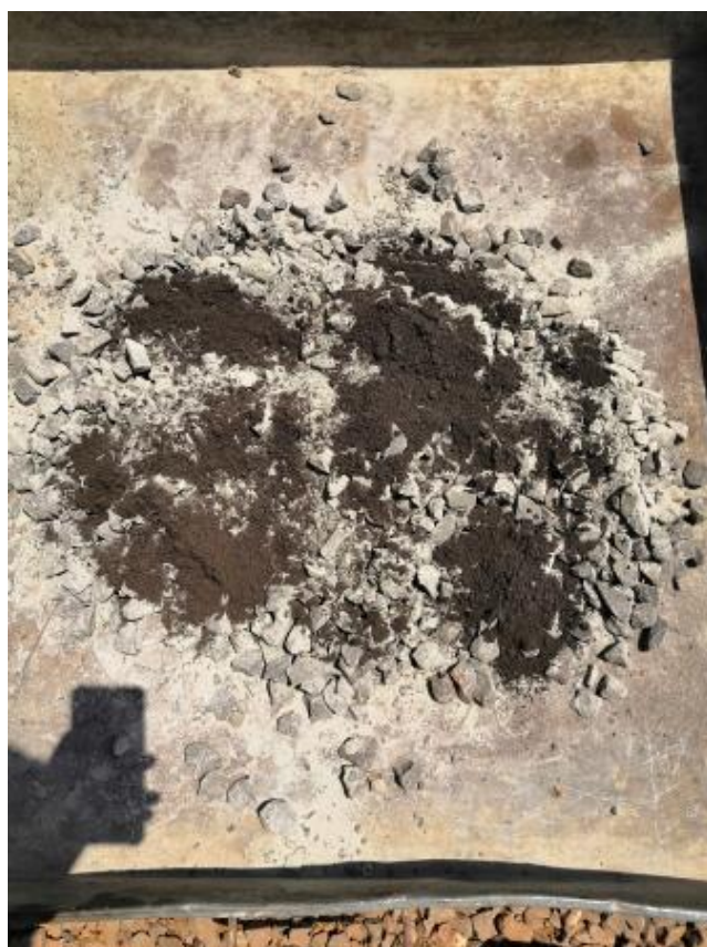
Figure-1d: Sludge mixed with cement and aggregates.
